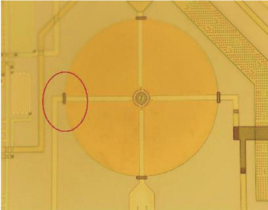
Photograph showing an SOI microhotplate (large circle) with a small micro-heater (12 micron radius) and integrated temperature sensor. DC power consumption is a few milliwatts at 300 C and tens of microwatts when operated in a pulsed mode. Red ellipse indicates very accurate back etch with alignment mark.
