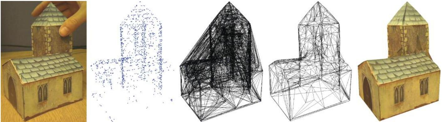
Left to right (a) Object rotated by hand in front of camera. (b) Point cloud obtained from on-line structure from motion estimation followed by bundle adjustment. (c) Delaunay Tetrahedralisation of point cloud, partitioning the convex hull into tetrahedra. (d) Carved mesh obtained from recursive probabilistic tetrahedron carving. (e) Texture-mapped surface mesh.
