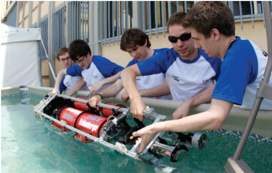
The team lowers Red Herring into the salt-water ballasting tank provided by the Nato underwater research centre in Italy.
