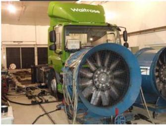
Dynamometer testing of Diesel-CNG dual fuel vehicle performance and emissions
