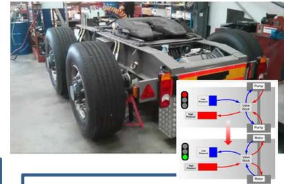
Hydraulic regenerative braking system for urban delivery vehicles
